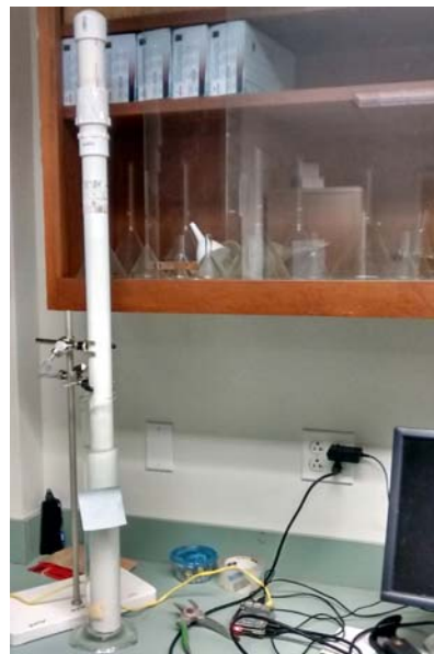
Figure 3. The experimental set-up for the artificial well comparison tests. The Solinst Barologger® is in the corner inside of the nylon sheath. The Disto, FTP, and Solinst Levelogger® are inside the well, and the Pi 2B is at the nexus of all of the cables in the bottom of the image.
